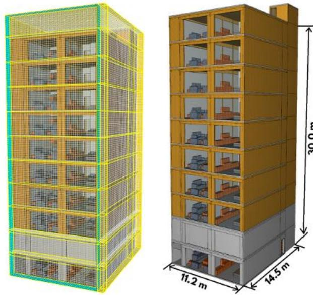
Figure 24: FDS model multi-storey CLT building (Hayajneh & Naser, 2023)
