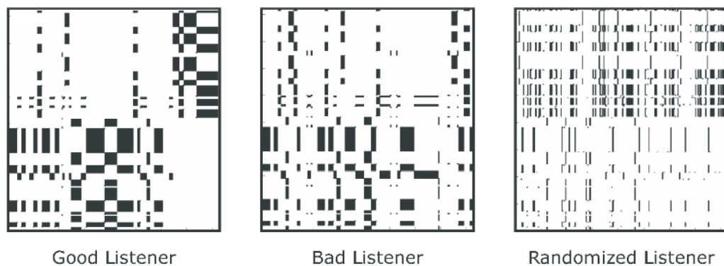
Figure 3.1: Cross-recurrence plots comparing eye gaze of speaker and different types of listeners adapted from Richardson and Dale [75]. The horizontal axis captures the gaze of the speaker and the vertical that of the listener. A good listener here has good alignment with the speaker while a bad listener is not as well aligned. This can be seen by the low amount of diagonal lines that can be drawn in the plot for the bad listener compared to the good listener. There is worse alignment between the speaker and a randomized listener compared to the other two listeners as can be seen in the small amount of black in the plot and no diagonal lines.
