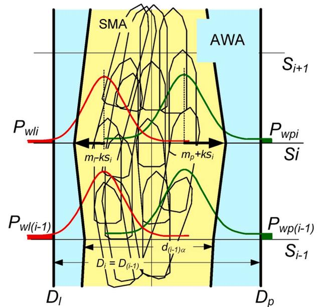
Fig. 3. Probabilistic method of defining the safe manoeuvre area (SMA) and the probability of ship outside the available water area (AWA).
