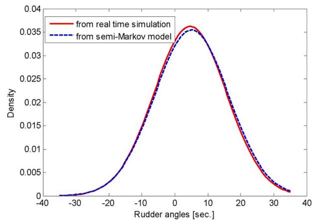
Fig. 18. Comparison of rudder distribution between the real time simulation and new model.
