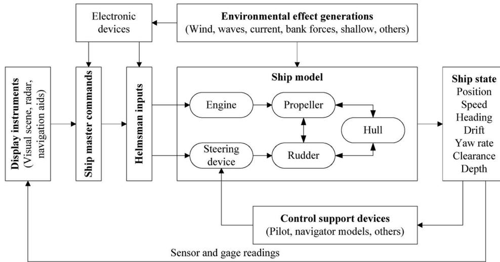
Fig. 1. A simplified ship-handling simulator.
