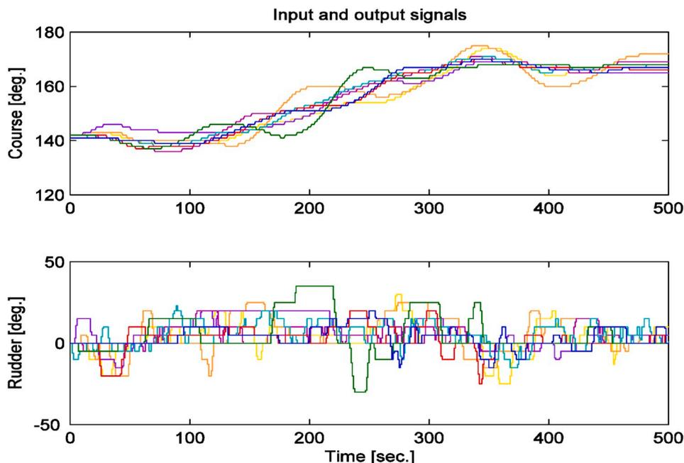
Fig. 14. Measured rudder angles in calm environmental condition for total 15 real time simulation trials.
