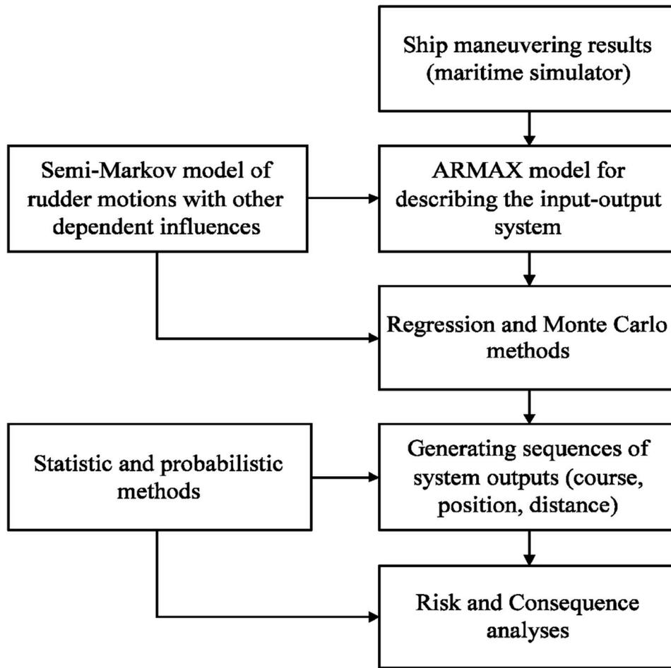
Fig. 12. General procedure for created ships performance model.
