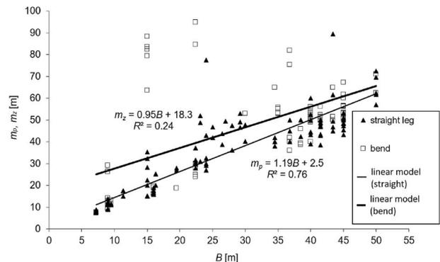
Fig. 9. Linear relation of mean width of manoeuvre area for straight waterways ( $m_p$ ) and bends ( $m_z$ ) to the ship's breadth ( $B$ ).
