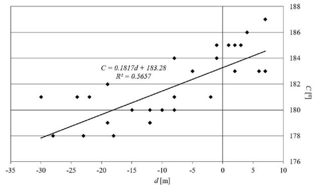
Fig. 6. Linear correlation between distance from the waterway centre ( $d$ ) and ships course ( $C$ ) for one investigated simulation waterway section presented on Fig. 6.
