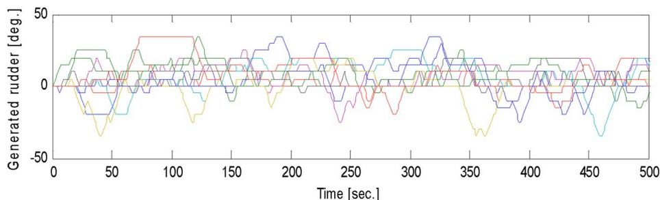
Fig. 17. An example of sequences of generated rudder angles from the semi – Markov model.
