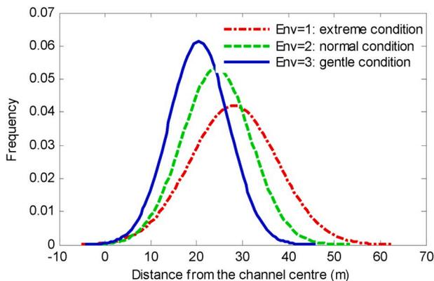
Fig. 4. Density function of distance from the centre of the channel fitted with normal distribution (in starboard side).
