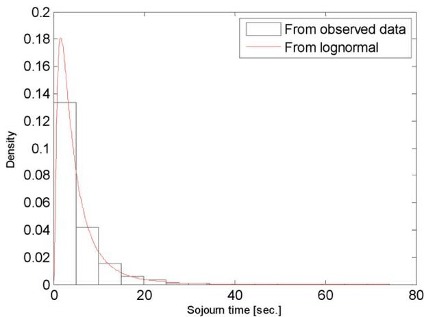
Fig. 16. An example of distribution of the sojourn time fitted with lognormal distribution.
