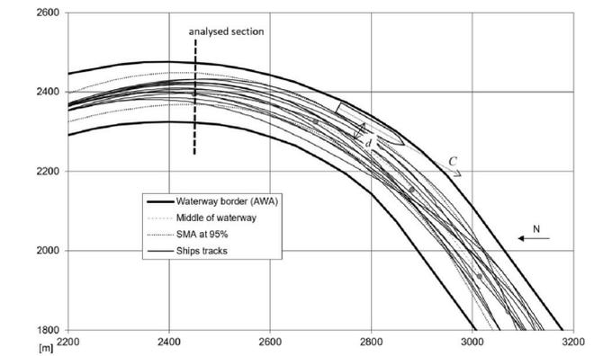
Fig. 5. Waterway area and 15 example ships tracks used for determining the relation between distance from the waterway centre ( $d$ ) and ships course ( $C$ ).
