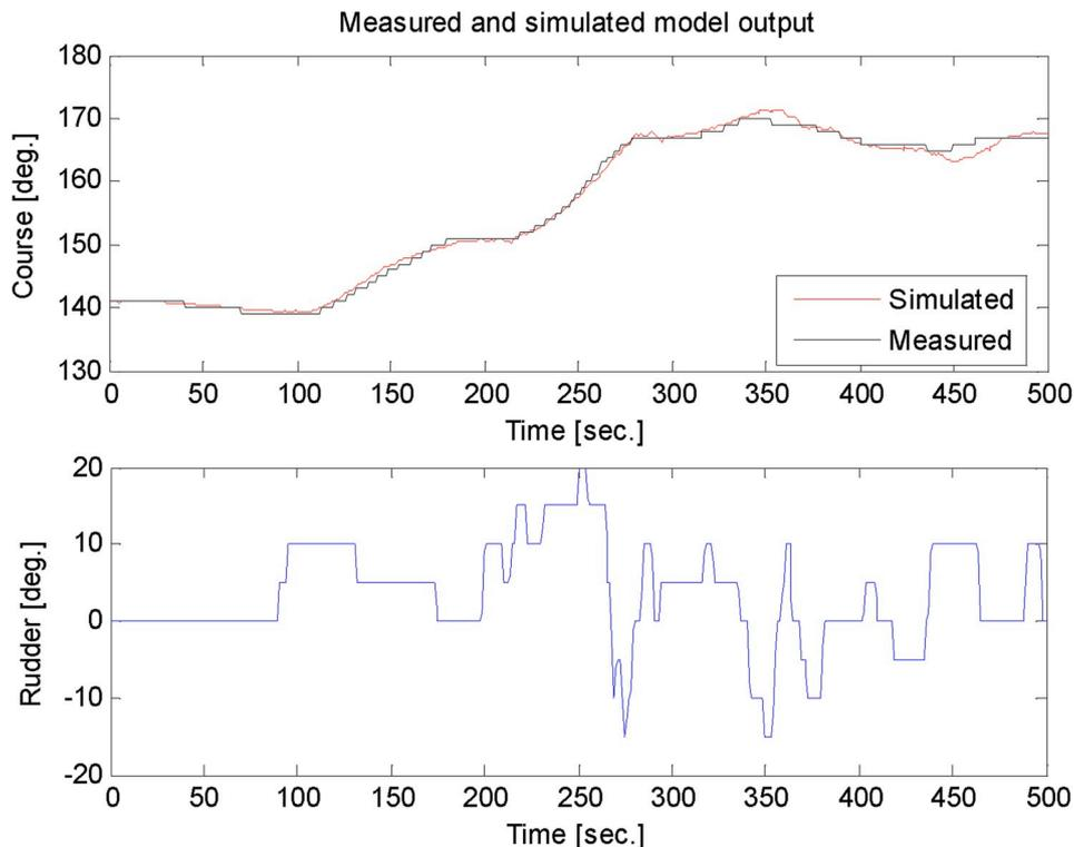
Fig. 20. Comparison between simulated and measured courses.
