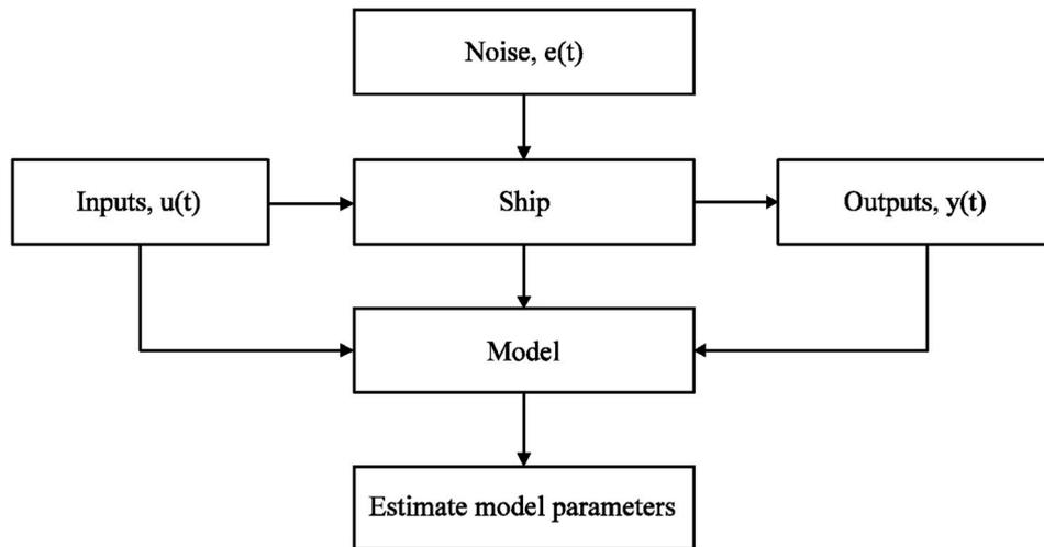
Fig. 13. Simplified model of ship dynamic.
