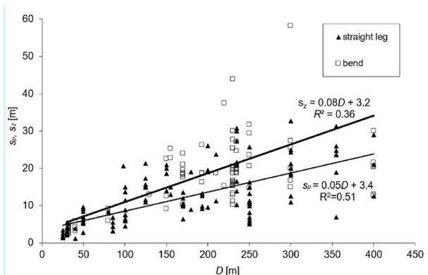
Fig. 10. Standard deviations on straight legs ( $s_p$ ) and bends ( $s_z$ ) dependence of available waterway width ( $D$ ).
