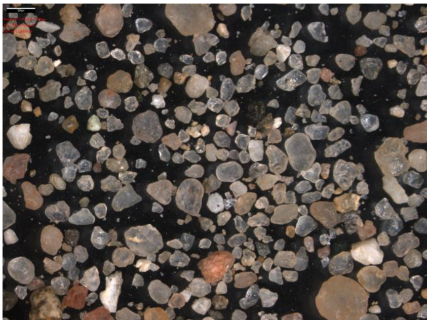
FIGURE A-4: SAMPLE STERKSEL FORMATION (B320 – M13), GRAINS SEPARATED
