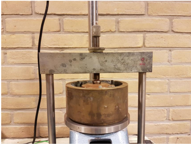
FIGURE A-14: CLOSE UP INSTALLED OEDOMETER MOULD
