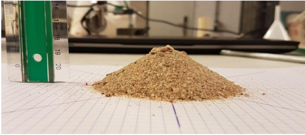
FIGURE A-8: ANGLE OF REPOSE MEASUREMENT OF HEIGHT
