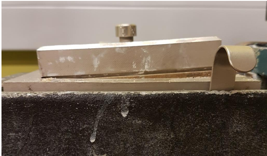
FIGURE A-27: TOP CAP TILTING DURING LOADING
