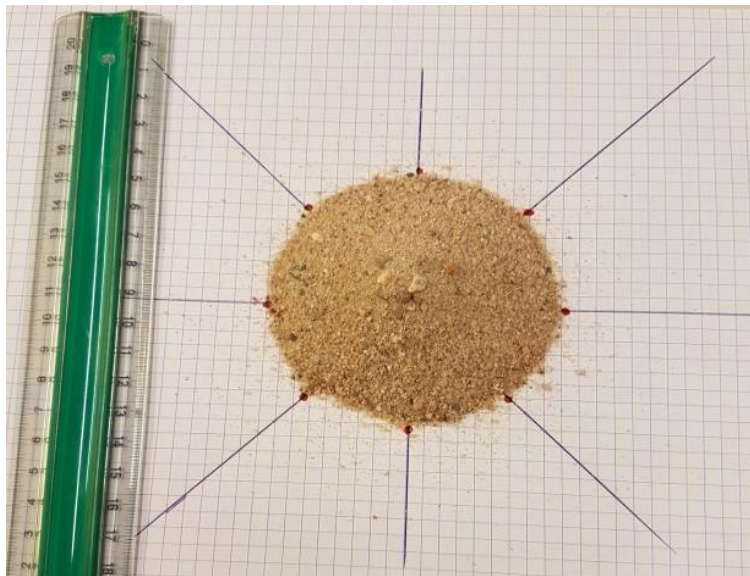
FIGURE A-6: ANGLE OF REPOSE MEASUREMENT
