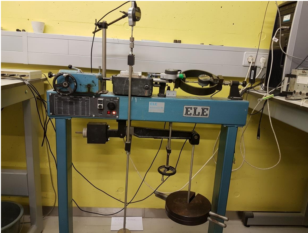
FIGURE A-25: PHOTOGRAPH DIRECT SHEAR APPARATUS, SIDE VIEW
