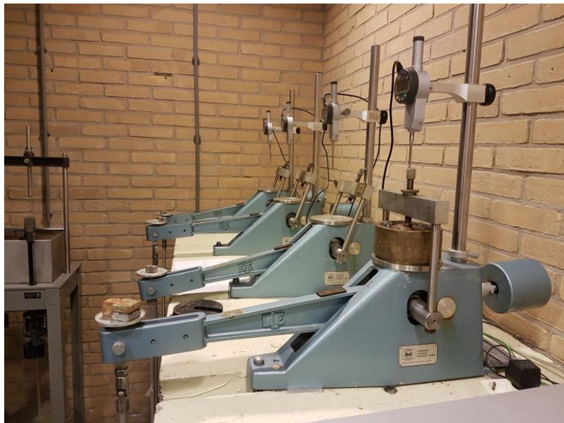
FIGURE A-13: OEDOMETER SET-UP
