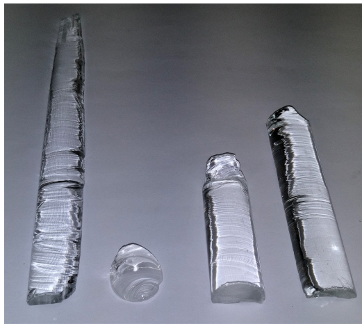
(a) Fractured rods ends belonging to Column 5.
