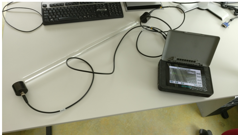
Figure 2.2: Determining the Young's modulus of a borosilicate glass rod using ultrasonic pulse velocity testing.
