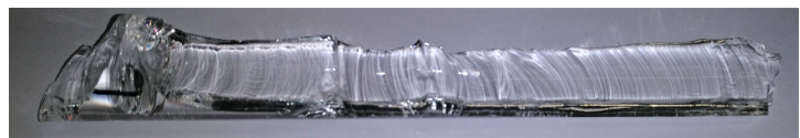
(b) Fracture from Column 18 where the Wallner lines show flexure cracks from different origins which propagate in different directions.
