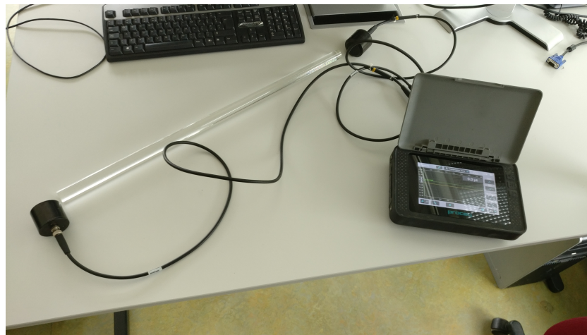
Figure B.5: Determining the Young's modulus of a glass rod using ultrasonic pulse velocity testing.
