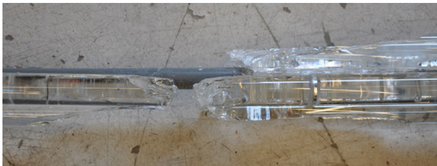
Figure 2.6: The failure pattern of a specimen of configuration C_1 [4].
