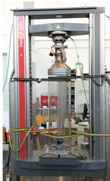
(b) The final test setup including a 5 mm thick polycarbonate tube as safety measure.
