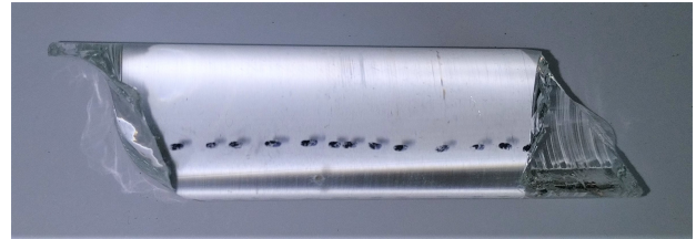
(c) Fracture expected to be due to twist of Column 2.
