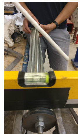
Figure 2.12: Initial twist in one of the Bend & Break columns.
