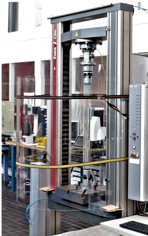
(a) The first try-out for the test setup with 2 mm thick sheets of acryl glass bend around the column as safety measure.
