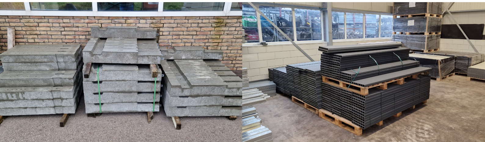
figure 4: concrete foundation (l) and recyclable fibre reinforced plastic foundation (r) (own, 2022)
