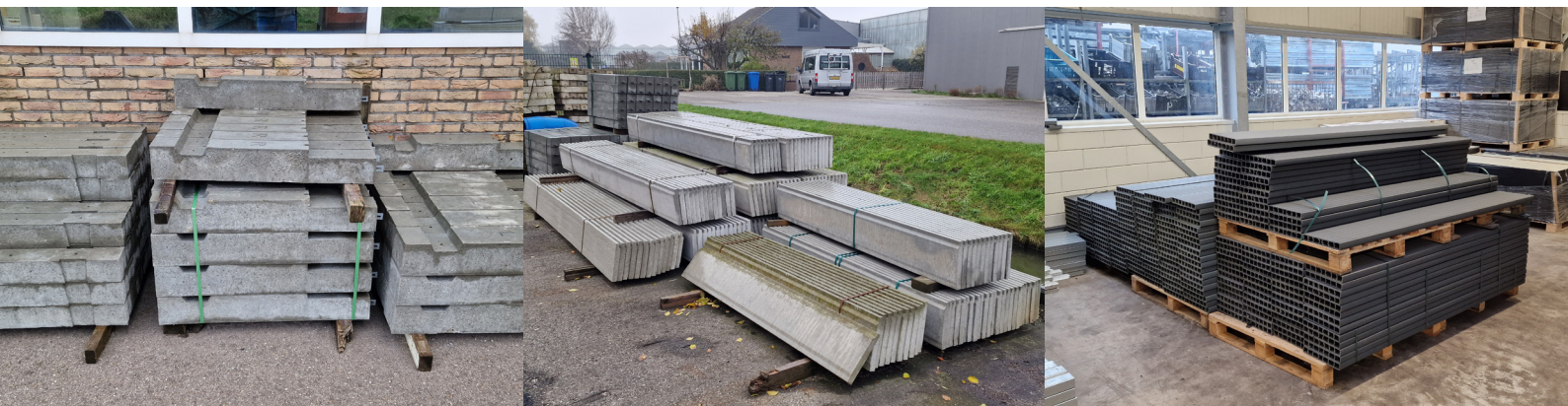
figure 71: concrete dollies (l), concrete slabs (m), and fibre reinforced slabs (r) (own, 2023)
