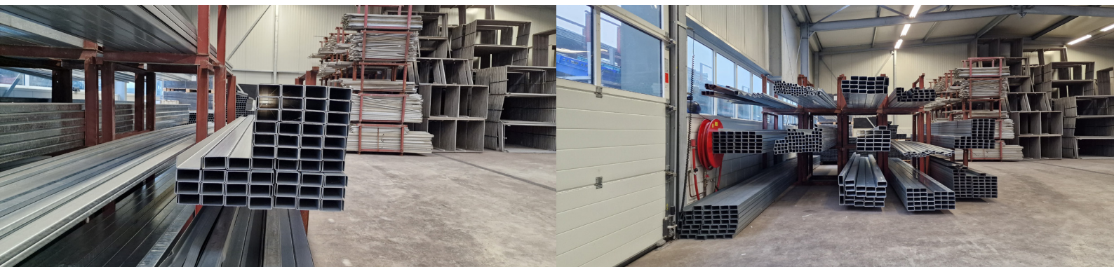
figure 69: magnelis RHS sections (l) and the variety of available magnelis profiles (r) (own, 2022).
