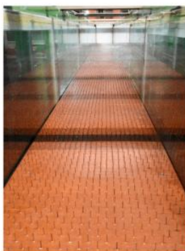
Roughness 4 Small nails, high density k_s = 10.0 mm
