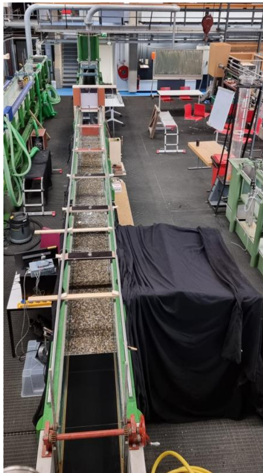
Figure 2.4: Top view dam-break wave test set-up with in the back the reservoir, halfway the flume the gate opening mechanism, in the downstream part of the flume 6 ADMs, in the front on the left side the Data Acquisition System and in the front on the right the tent for video recording and taking photos
