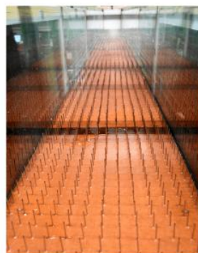
Roughness 5 Long nails, low density k_s = 26.0 mm
