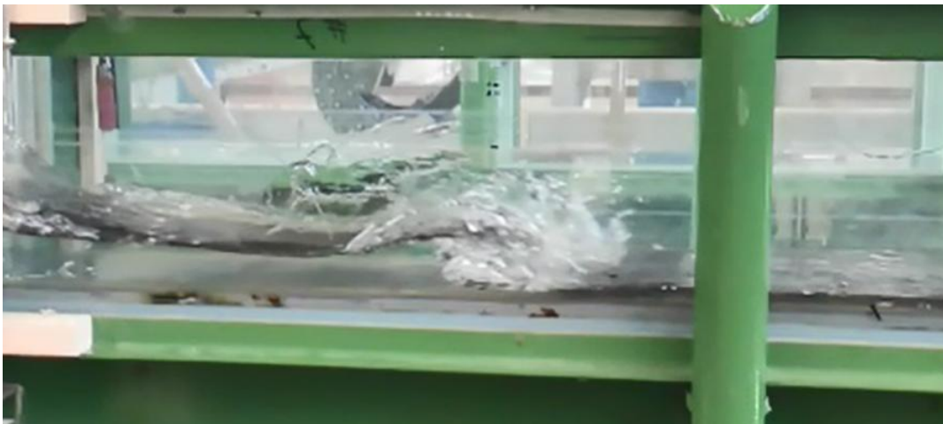
Figure 4.1: Breaking bore after releasing the water from the reservoir into the downstream channel 0.7 m downstream of the gate for a Ref (smooth) wet bed 25 mm test (flow from left to right), test W25R0T9 (Table 2.2)
