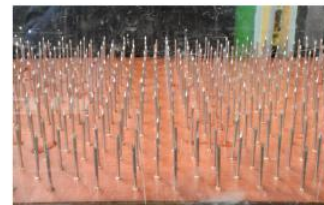
Roughness 7: Large nails, high density ( k_s = 48.0 mm)
