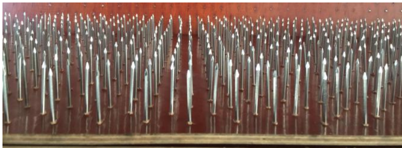
Figure 2.8: Side view of artificially created roughness R7 (long nails, high density) k_s = 48 mm
