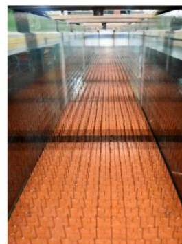
Roughness 6 Small and long nails, high density k_s = 27.5 mm
