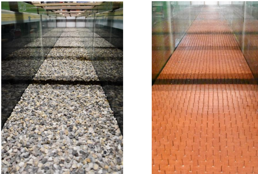
(a) Naturally created roughness R2 (large gravel d_{50} = 5 mm) k_s = 6.0 mm
