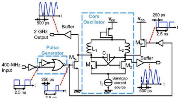
Fig. 6. Injection-locked transmitter for narrowband FM [11].
