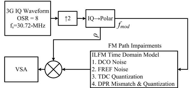
Fig. 9. System test bench of DFC employing ILFM.
