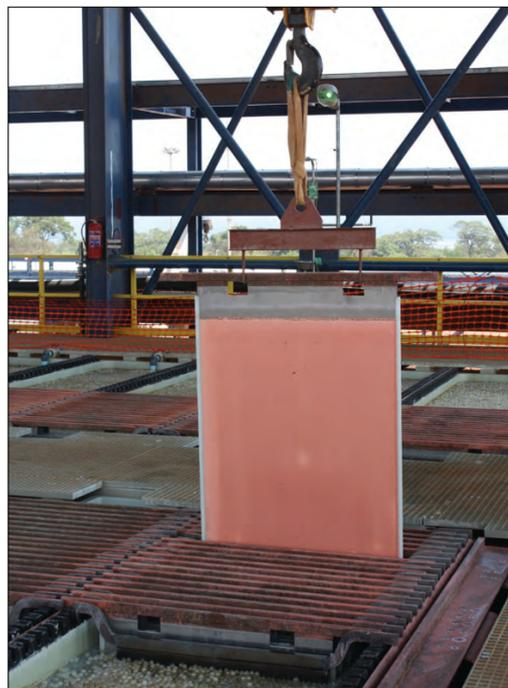
**Figure 3.6:** Copper cathode from the heap leach operation (Wimberley et al., 2011)
