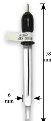
**Figure 4.5:** Small size Ag/AgCl reference electrode with 3 M NaCl electrolyte
