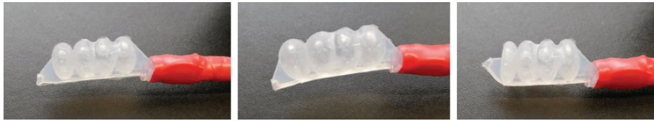
Figure 22: Fluid pressure in a silicone structure
