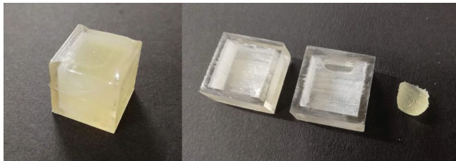
Figure 42: support structure printed inside the cube fluid environment
