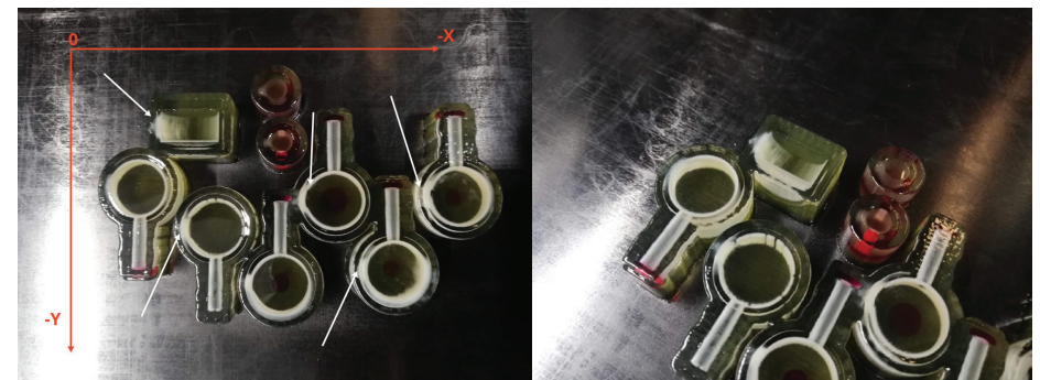
Figure 56: improperly cured resin prominent along -y axis
