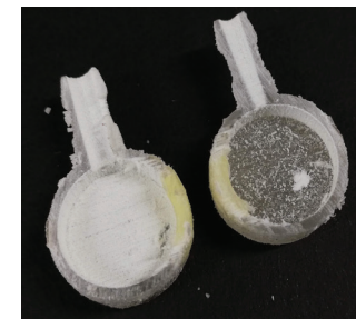
Figure 50: No imperfections or collapse can be observed on the soft membrane.
