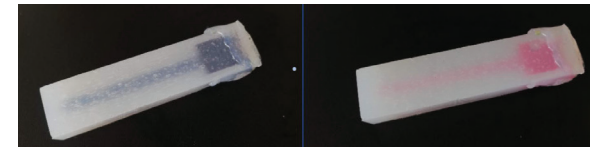
Figure 20: temperature reacting appearance, with the use of heat reactive colouring fluid
