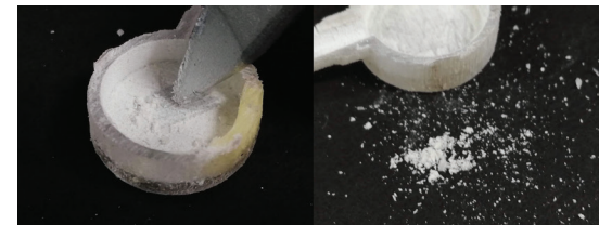
Figure 34: white flakes scraped off rigid material (transparent), printed in contact with fluid
