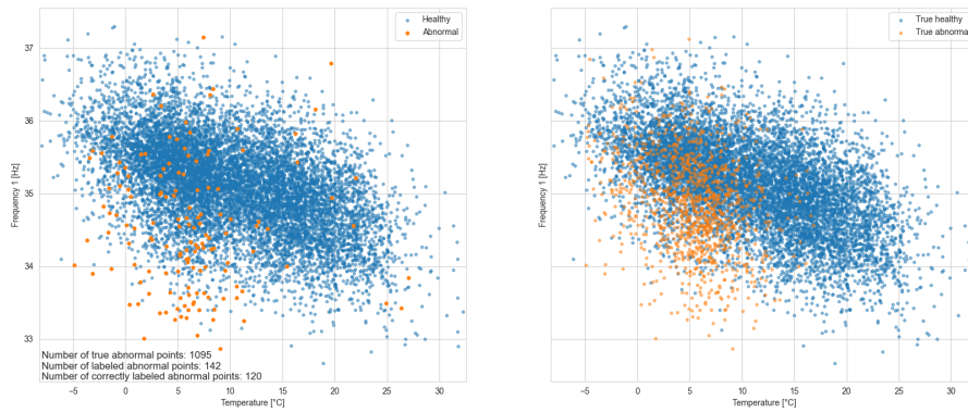
GMM-based anomaly detection results for 150 mm gradual settlement and 3% Sudden stiffness reduction - Months: 3
