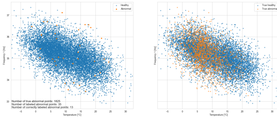
GMM-based anomaly detection results for 150 mm gradual settlement and 3% gradual stiffness reduction - Months: 5
