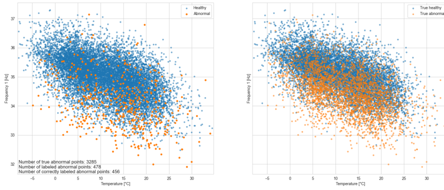
GMM-based anomaly detection results for 150 mm gradual settlement and 3% Sudden stiffness reduction - Months: 9
