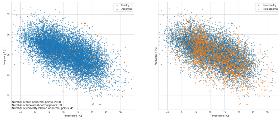
GMM-based anomaly detection results for 150 mm gradual settlement and 3% gradual stiffness reduction - Months: 8
