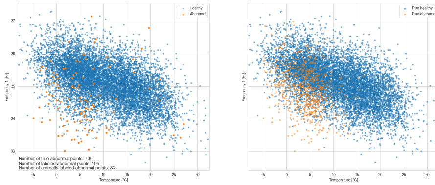
GMM-based anomaly detection results for 150 mm gradual settlement and 3% Sudden stiffness reduction - Months: 2
