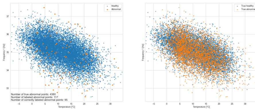
GMM-based anomaly detection results for 150 mm gradual settlement and 3% gradual stiffness reduction - Months: 12
