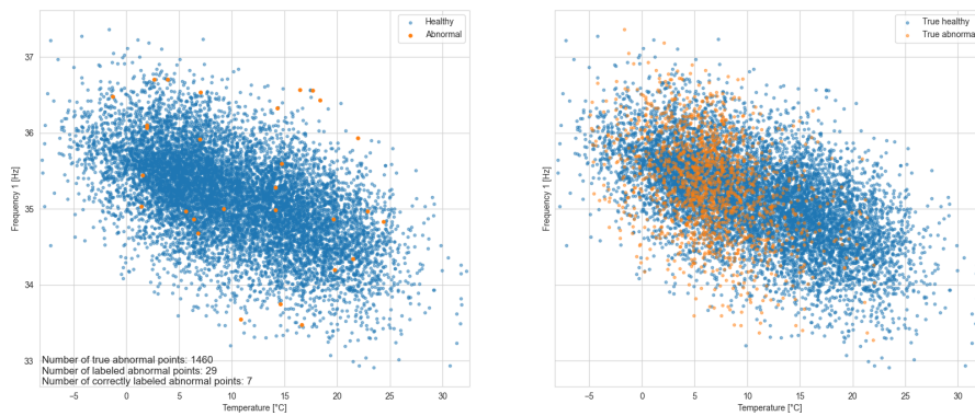
GMM-based anomaly detection results for 150 mm gradual settlement and 3% gradual stiffness reduction - Months: 4
