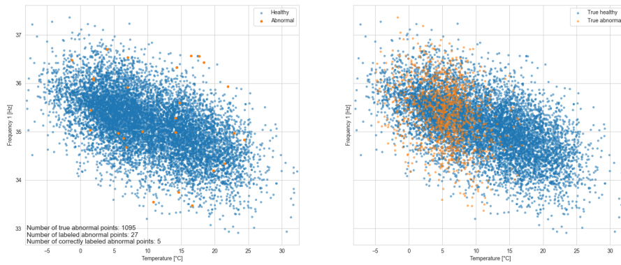
GMM-based anomaly detection results for 150 mm gradual settlement and 3% gradual stiffness reduction - Months: 3
