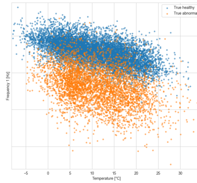
GMM-based anomaly detection results for 10% sudden stiffness reduction - Months: 12
