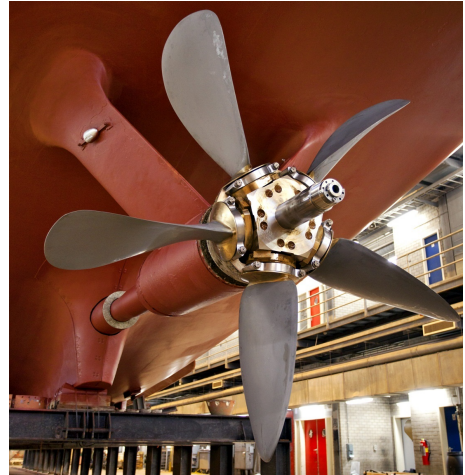
Figure 1.2: Composite propeller of the Alkmaar-class minehunter (Photo: Airborne Composites BV).
