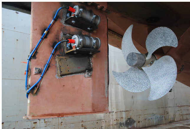
Figure 6.14: Portside rudder with the cameras and the composite propeller with the speckle pattern.
