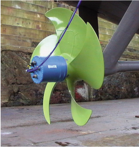
Figure 1.1: The composite propeller of the Triton (Photo: QinetiQ).
