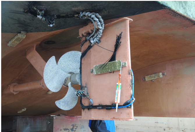
Figure 6.15: Lights on the rudder and hull and routing of the cables.
