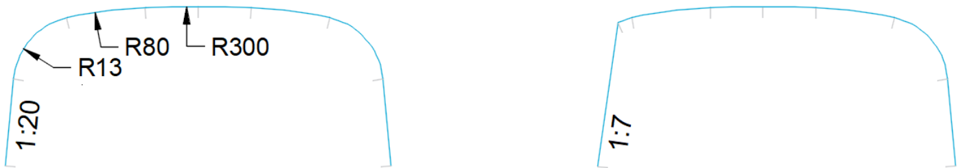
Figure 6 - An example horizontal profile; a top view from the track center line, starting in the origin
