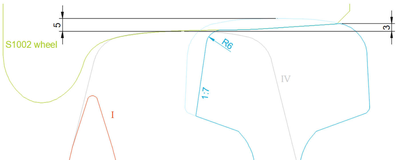
Figure 60 - Kloos crossing cross-section I: with the wheel profile (green), nose rail (orange) and wing rail (blue)
