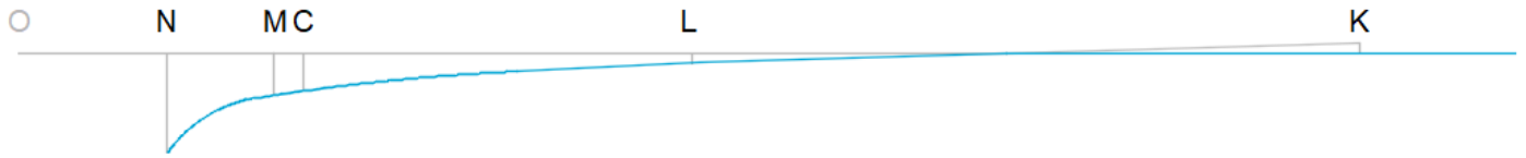
Figure 69 - German nose profile, consisting of semi ellipses
