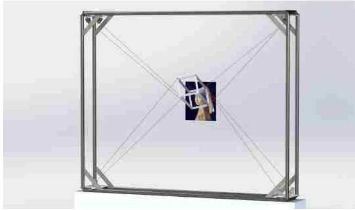
Fig. 1: CAD rendering of proposed cable robot CaRISA depicted scanning Vermeer's Girl with a Pearl Earring (picture CC-BY-SA 3.0 Unported License).
