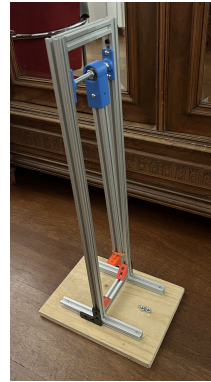
Figure 3: Picture of the pendulum setup
