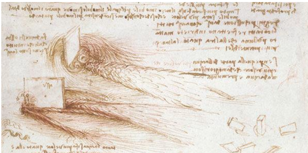
Figure 4-2: A rigid obstacle in flowing water creates wake turbulence, a fact noted and sketched by Leonardo da Vinci in 1509 Bingham (2007)
