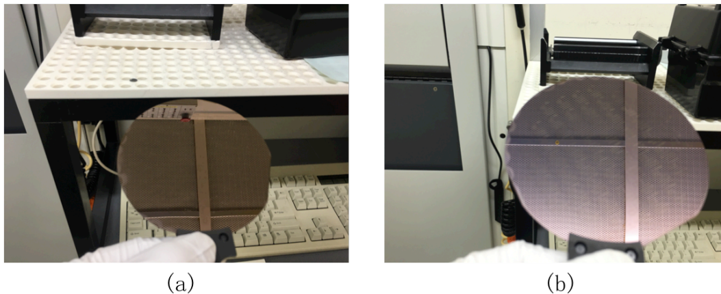
Figure 4.12: TiN surface conditions. (a) surface color after metal deposition; (b) surface color after Tepla oxygen plasma photoresist removal
