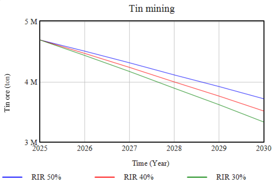
Figure 17: Tin reserve depletion with different Recycling input rate (RIR) extracted from the model. (Created with the software Vensim)
