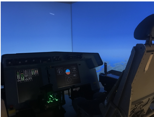
Fig. 5 Fixed-base simulator in aircraft configuration
