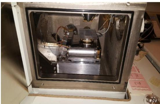
FIGURE 8: AN IMAGE OF THE SAMPLE CHAMBER WITH A THORN-SANDSTONE THIN-SECTION PLACED INSIDE.
