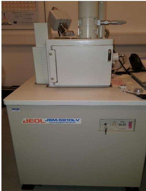
FIGURE 7: THE JEOL JSM-5910LV SCANNING ELECTRON MICROSCOPE.
