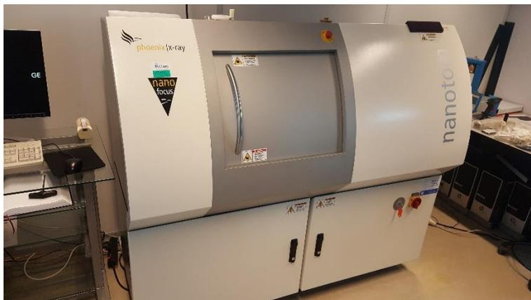
FIGURE 5: PHOENIX NANOTOM MICRO-CT SCANNER AT THE FACULTY OF GEOSCIENCE (TU DELFT).
