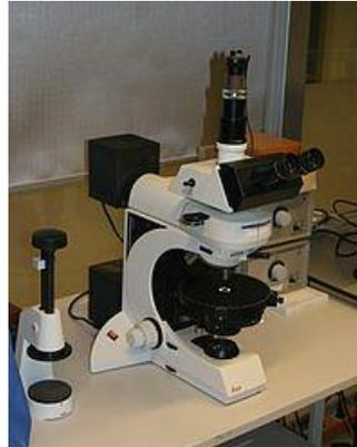
FIGURE 4: LEICA DM/LP POLARIZATION OPTICAL MICROSCOPE.
