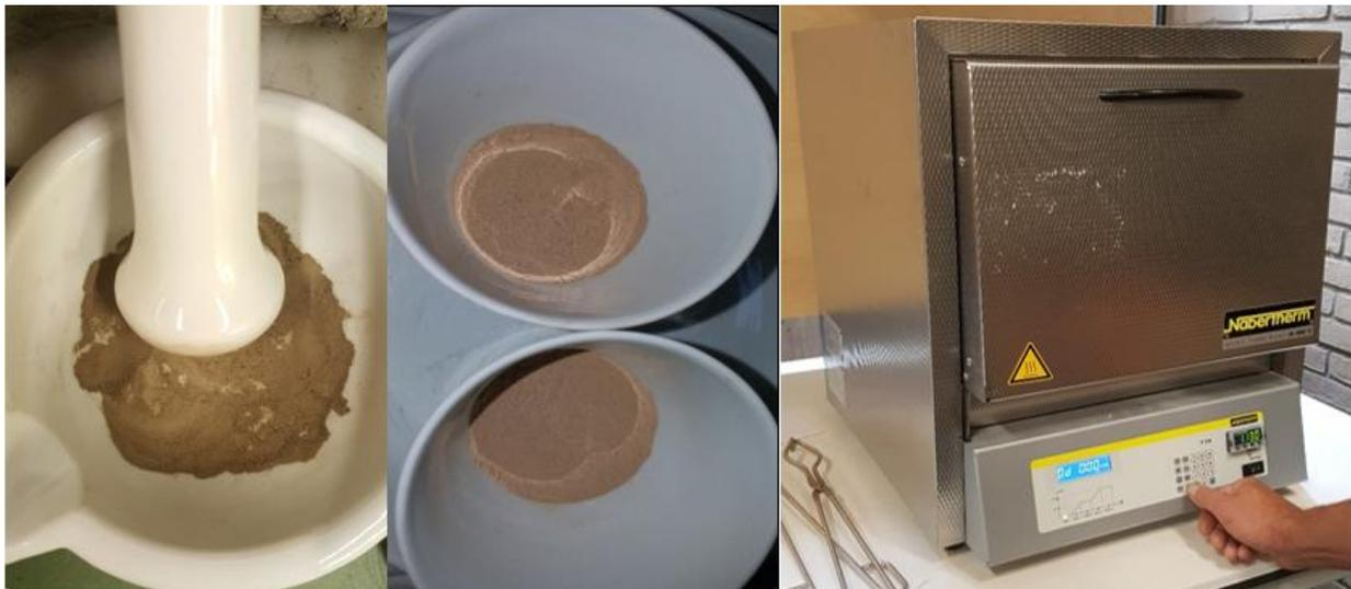
FIGURE 6: POWDERED ROCK SAMPLE (LEFT), TWO PORCELAIN DISHS WITH ROCK POWDER (CENTER) AND BURNING OVEN (RIGHT).
