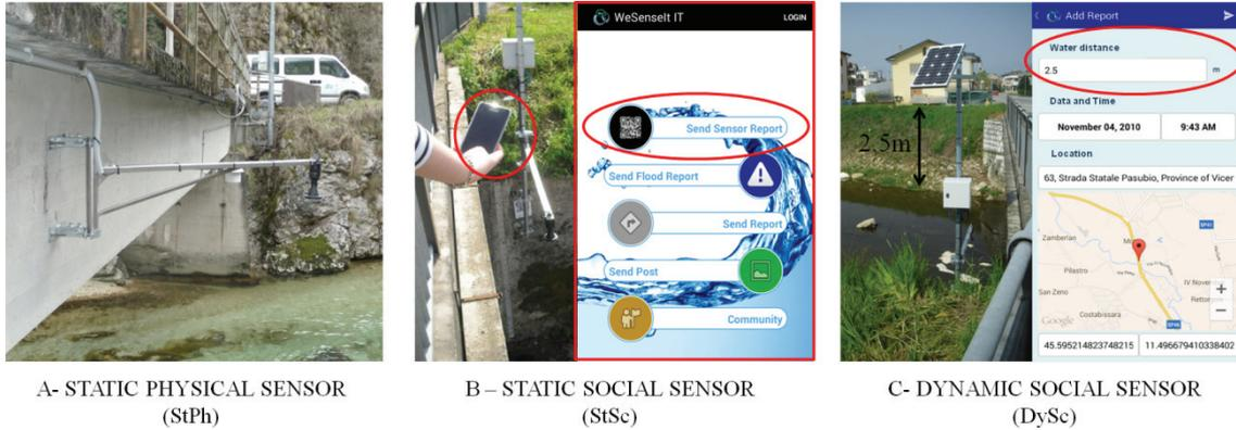
Figure 1.7. Sensor classification used in this thesis
