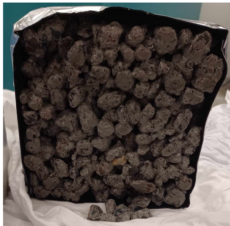
Figure 5.6: Loosening of aggregates from Mix 2 after 28FT cycles.
