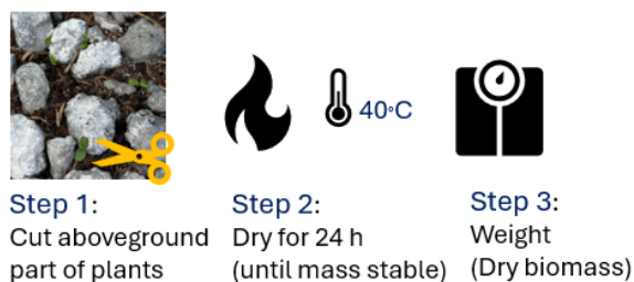
Figure 4.17: Test set up for measuring dry biomass of plants.
