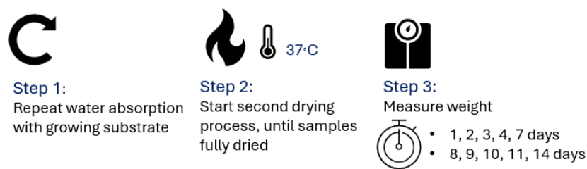
Figure 4.16: Water retention process.
