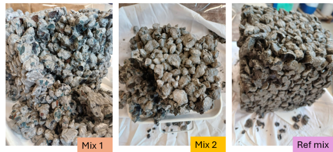
Figure 5.1: Breaking points of concrete samples after compressive strength test.
