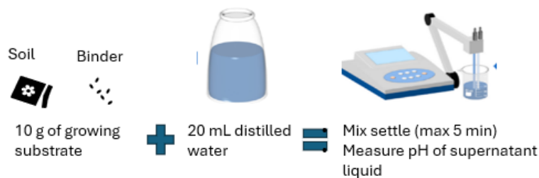
Figure 4.12: Test set-up for measuring pH of the growing substrate.
