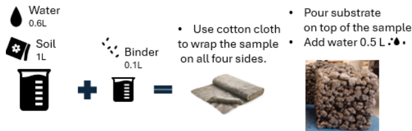
Figure 4.8: Process of water pouring method with cotton cloth.
