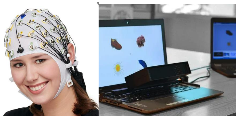
Figure 1. Left: EEG cap. Right: Laptop with eye-tracking camera mounted on top of the keyboard.
