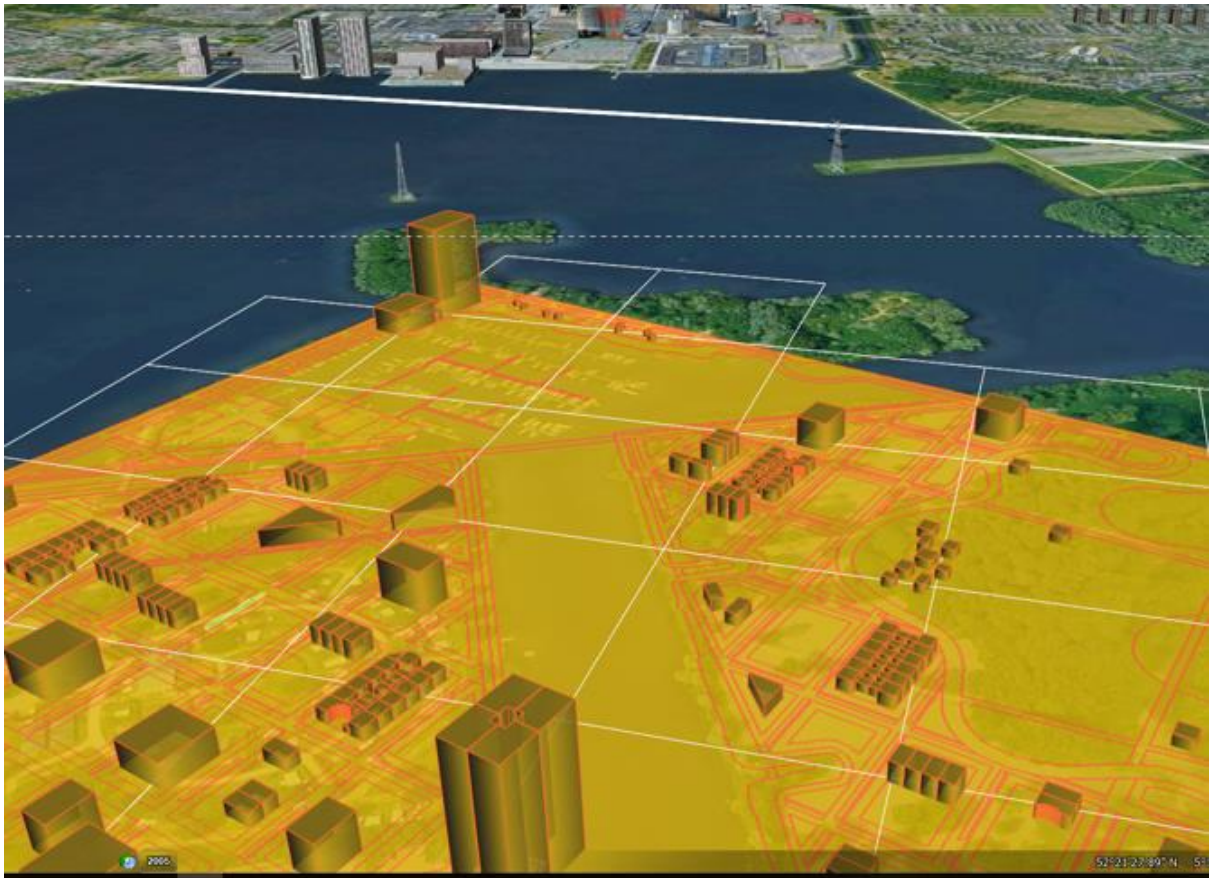
Figure 51: CityGML LOD1 Building model of the Floriade district, exported in KML by 3DcityDB Importer-Exporter and visualized in Google Earth
