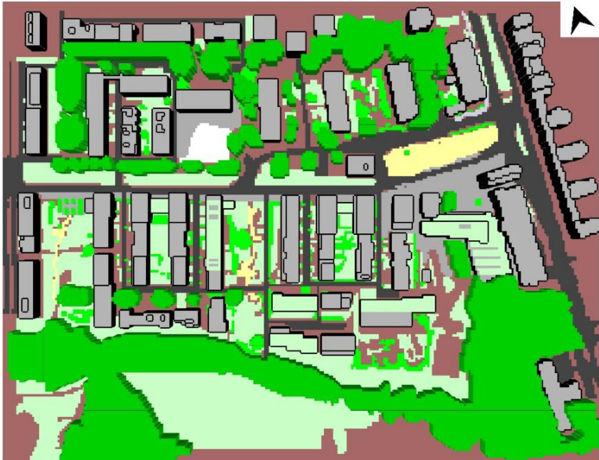
Figure 16: Model area displayed in SPACES editor. Buildings (grey), vegetation(green) and surface material colour coded (Source: Huttner, 2012)
