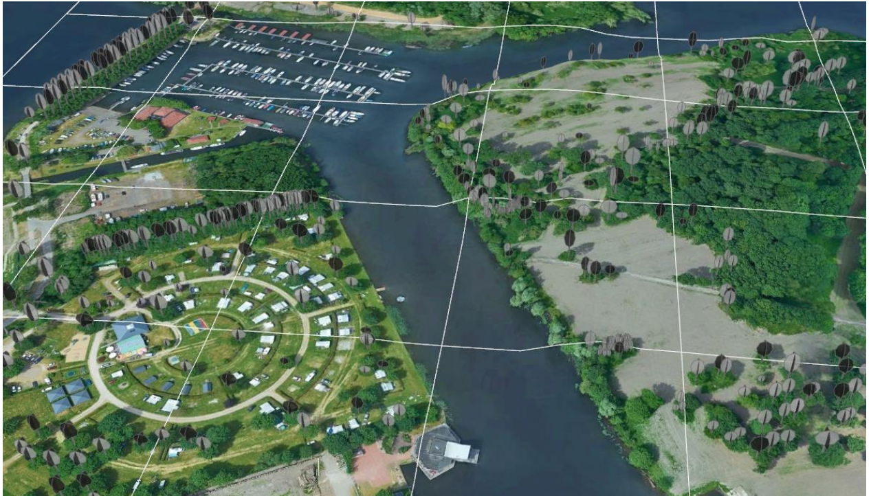
Figure 57: Vegetation module of Floriade CityGML model, exported as KML and visualized in Google Earth
