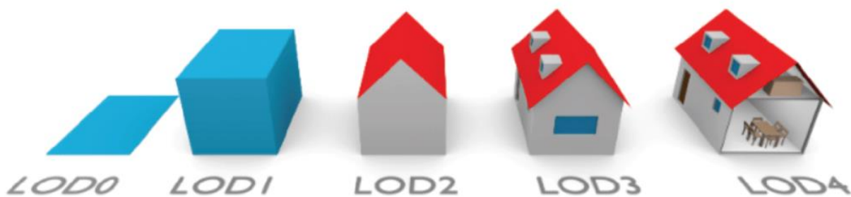
Figure 1: The 5 different CityGML level of details (LoDs) depicted on the Building module, Source: (Biljecki, 2016).
