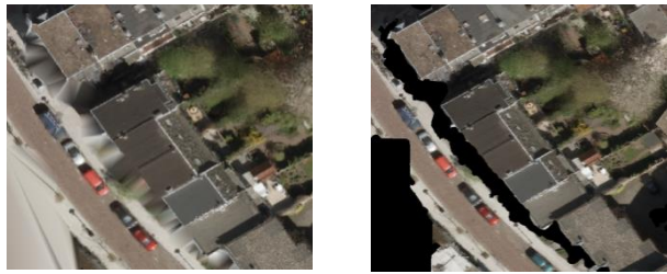
a. An occluded image b. A clean image Figure 10. Removing the occluded areas to provide clean training samples
