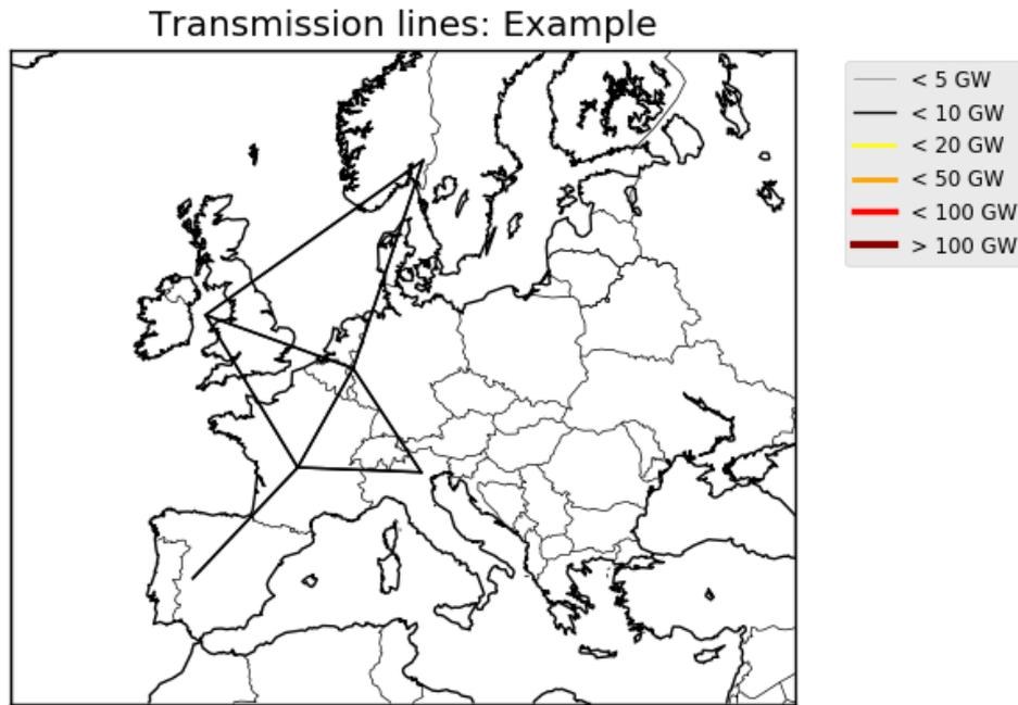
**Figure 3.2:** Example of a linearised inter-regional transmission grid for Europe, modelled using Python. Transmission capacity is represented in GW, lines represent the linearised power flow from region to region.
