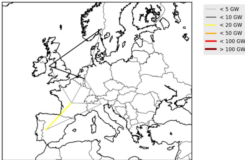
*Figure 5.3: Map of Transmission lines between regions, Reference Scenario. The lines represent the installed transmission capacity between the geographical centers of the regions, according to the copper plate model.*
