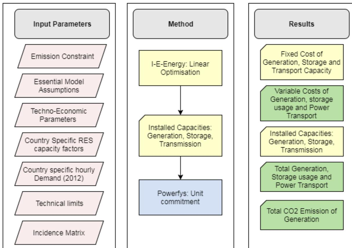
**Figure 3.3:** This flowchart describes the relation between input data, the modelling steps and the desired results. Input data is illustrated by red parallelograms, the results generated by only model I-E-Energy are illustrated by yellow cards, the results generated by both models are represented by green cards. The yellow and blue rectangles represent the models I-E-Energy and Powerfys, respectively
