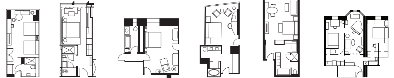
Marriott Marquis 4.2 x 9.2 m 40 m 2 Equinox Hotel 4.2 x 10 m 42 m 2 The Plaza 7.2 x 6.4 m 43 m 2 Aria Rooms & Suites Las Vegas* 5.2 x 9.6 m 48 m 2 Four Seasons Orlando* 4.5 x 12.5 m 55 m 2 Chelsea Hotel 8.4 x 7.8 m 74 m 2
