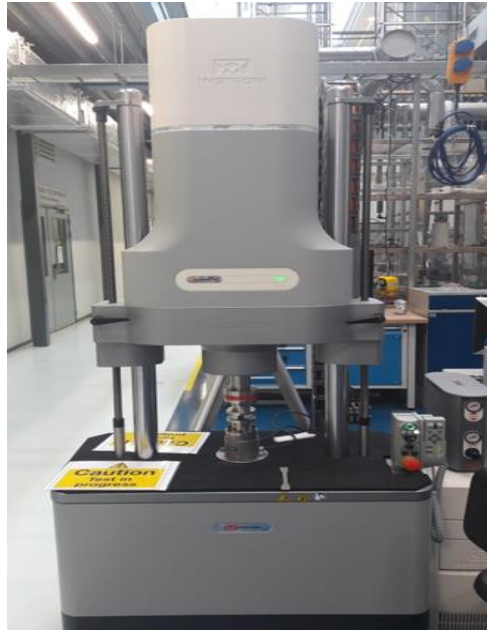
Figure 3.4 Instron Electropuls E10000 used for fatigue testing.
