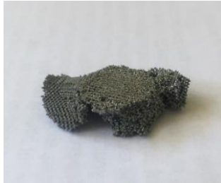
Figure 5.7 Compression specimens after testing (a) Vector based and (b) STL based.
