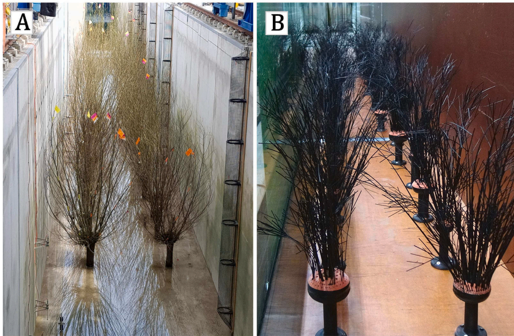
Fig. 4. (A) The real-scale experiments with the 50% density live trees, (B) the scaled experiments with 50% density 3D-printed trees (1:10 scale).
