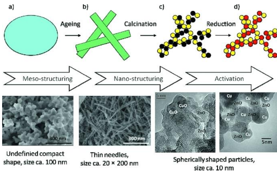
Figure 1.8 Simplified preparation scheme of Cu/ZnO catalyst from zincian malachite precursor and electron microscopy images of the different stages of preparation. 27
