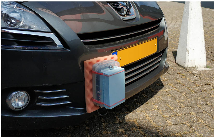
Figure 7.7: The front of the car with the MIMO radar system attached
