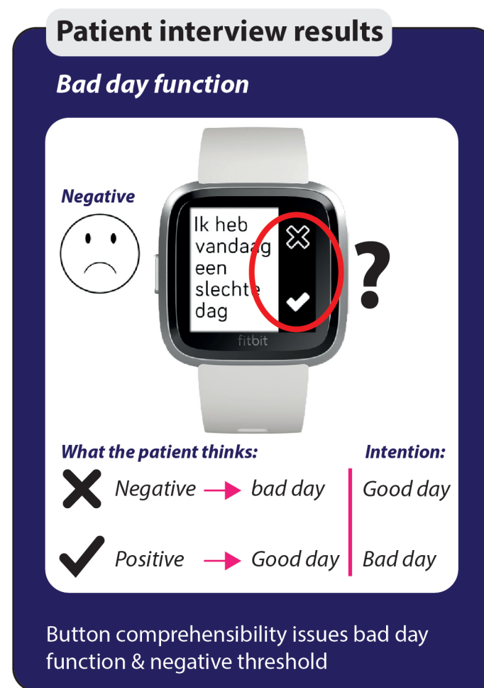
Image 62: Bad day function comprehensibility problems that were revealed during the user test interviews.
