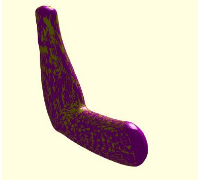
Figure 26. Overlapping Surface, Result of the Non-Rigid ICP. Yellow surface is the Deformed Source. Purple Surface is the Target Surface
