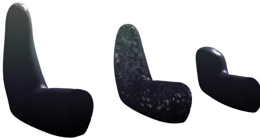
Figure 30. Resulting surfaces in direction of the first principal component (shape mode) of the General SSM. Left: -3 Standard Deviation, Centre: Mean Surface, Right: +3 Standard Deviation
