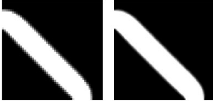
Figure 2.3: Optimized pipe geometries for a coarse and fine mesh that minimize viscous dissipation [1] using a Stokes flow model.
