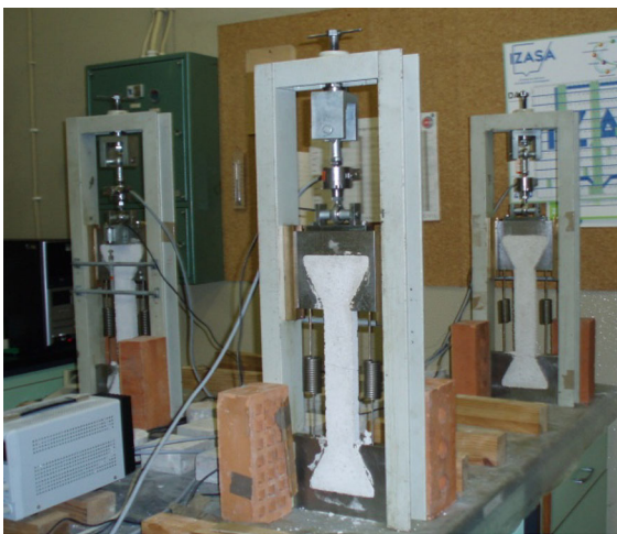
Fig. 11 Uniaxial restrained shrinkage test
