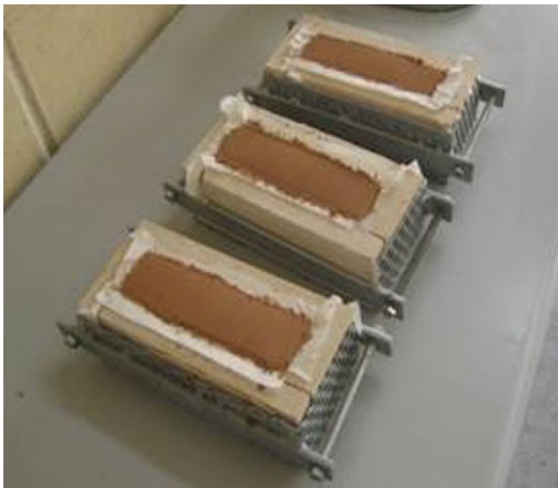
Fig. 7 Prismatic limestone moulds with crushed brick-air lime mortar cast in them [20]
