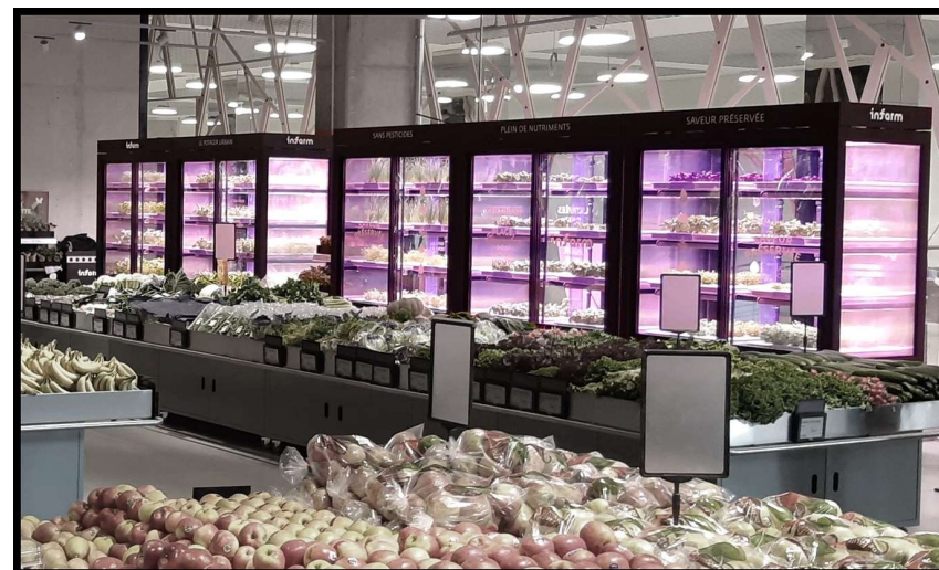
Fig. 22. Mini-PFAL in a supermarket. From Infarm (2020). Note: most of these supermarket integrations only keep the crops fresh as opposed to facilitating a complete growth cycle.
