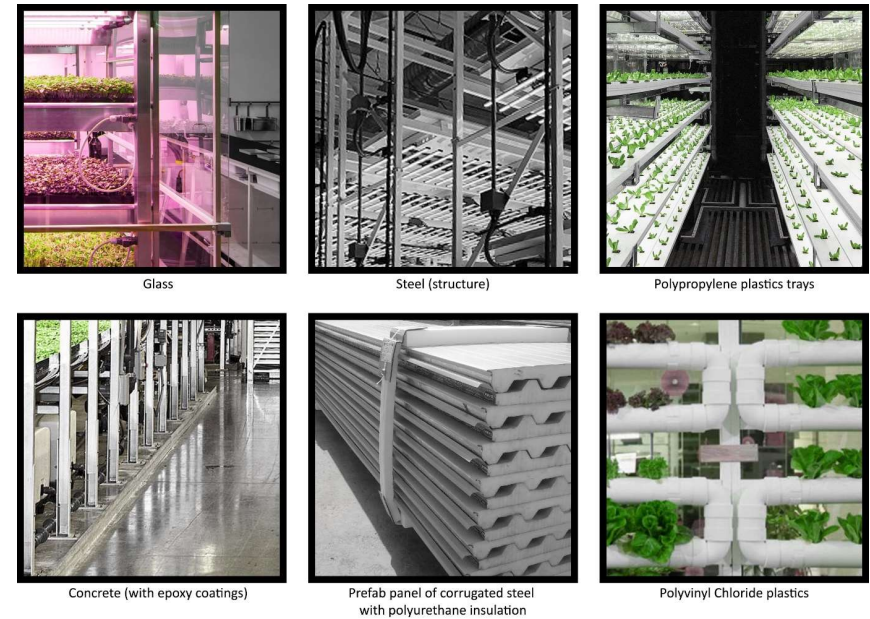
Fig. 27. Materials commonly occurrent in a PFAL.
