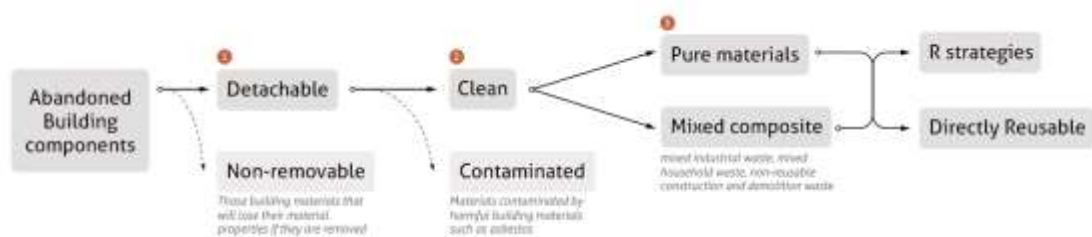
Figure 3 Classification of materials. Refer to the Amsterdam Cycle Monitor. Drawn by the author.
