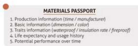
Figure 5 Information about the material that will be recorded on the MPs. Drawn by the author.
