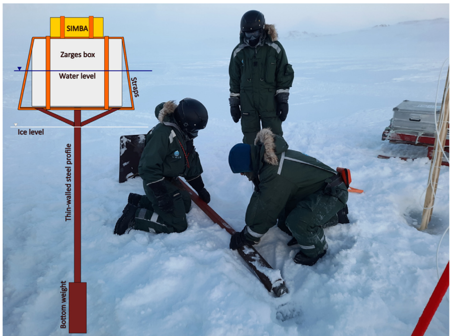
Fig. 10. Technical sketch and installation of the floating device, increasing the probability of a successful recovery of the SIMBA control box and attached wooden pile in the summer.
