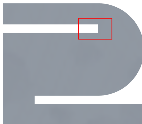
Figure 5.1: Geometry of the trapped vortex burner with the blunt shaped tip. The red box shows the focus location which will be studied with the first parameter.
