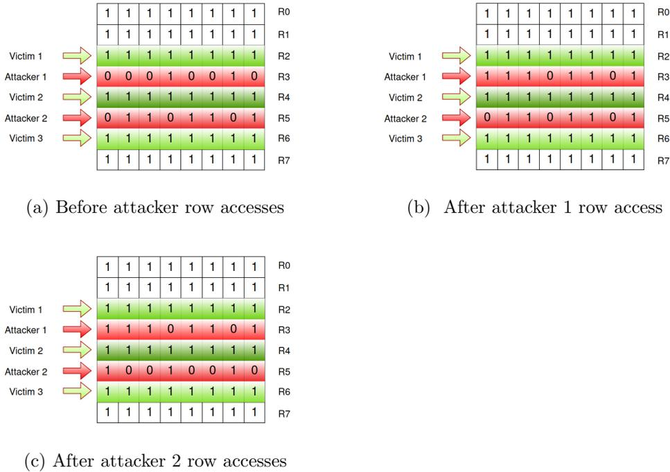
Figure 3.2: Attacker row content flipping during two-sided rowhammer
