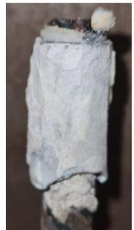
Figure 4-18: Corroded aluminium pipe
