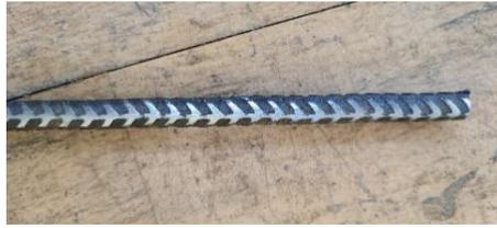
Figure 4-13 b: Sanded and cleaned rebar
