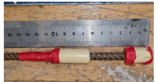
Figure 4-23 f: Fully completed rebar
