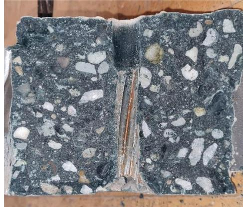
Figure 5-15 b: Spiral geometry imprinted in concrete matrix
