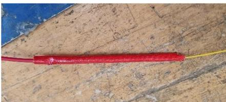
Figure 4-13 m: Spliced fibre (red) to pigtail (yellow)
