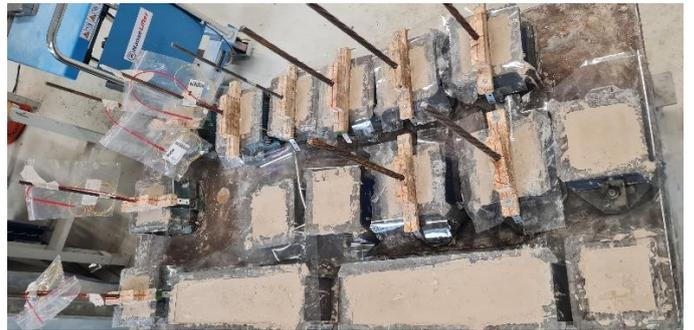
Figure 4-5 e: Plastic covered specimens after casting
