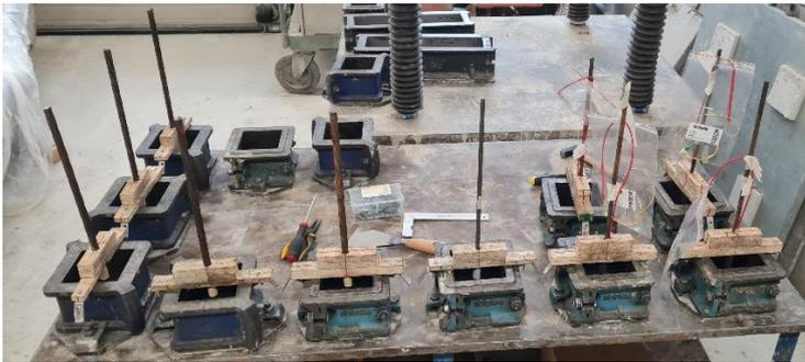
Figure 4-5 d: Prepared specimens just before casting
