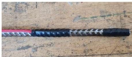
Figure 4-13 n: Wrapping DFOS unbonded region
