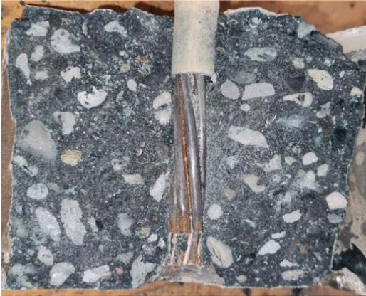
Figure 5-15 a: Cross-section prestressed reinforced AASC
