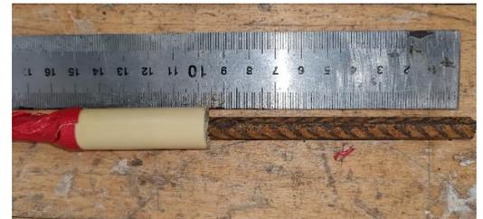
Figure 4-23 c: Top pipe: securing in place with tape
