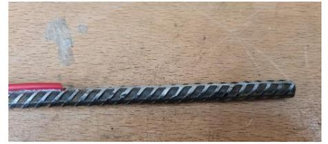
Figure 4-13 c: Attaching DFOS sleeve
