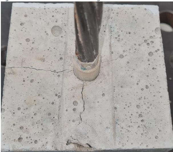
Figure 5-20f: Post test splitting failure crack formation (top)
