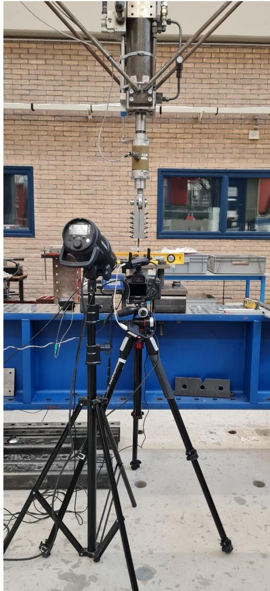
Figure 4-25: DIC camera setup
