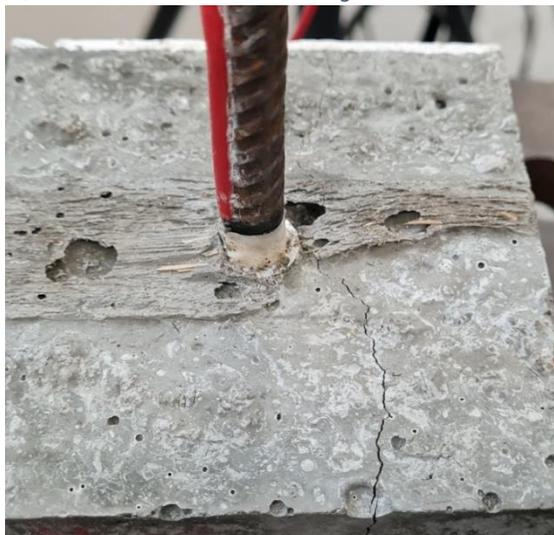
Figure 5-7f: Post test splitting failure crack formation (top)
