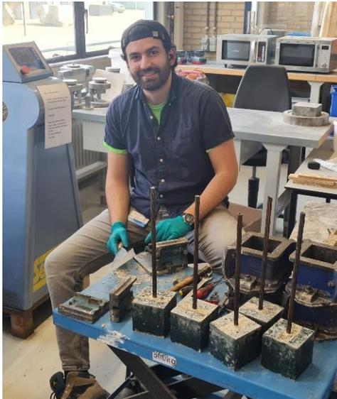
Figure 4-5 f: Demoulding AASC concrete 100mm sized cubes
