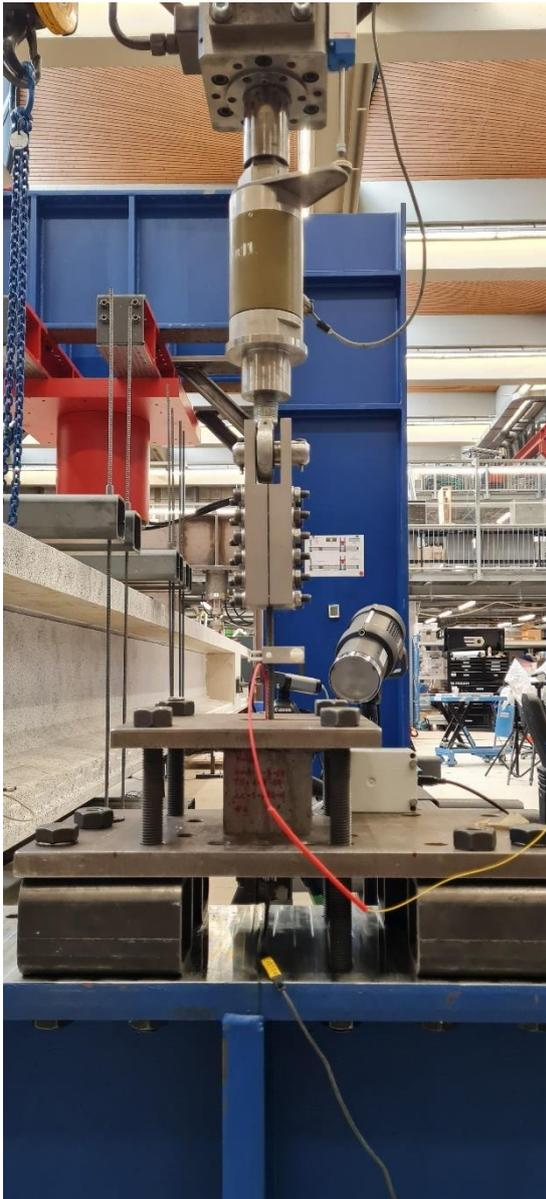
Figure 4-24: Pull-out test setup
