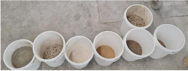
Figure 4-5 a: CC casting weighed materials; sand, aggregate and GGBFS
