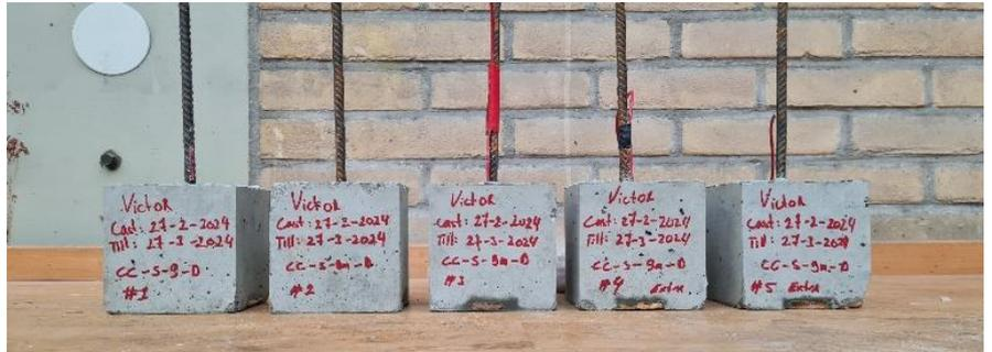
Figure 4-5 g: Labelling concrete specimens after demoulding (ME #3 CC)
