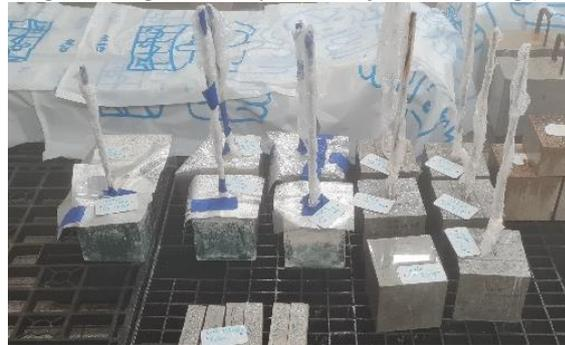
Figure 4-5 h: Moisture cured specimens (fog room). AASC specimens are covered, CC fully exposed
