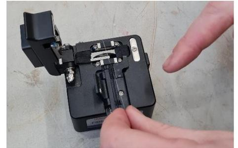
Figure 4-13 i: Placing fibre in cleaver
