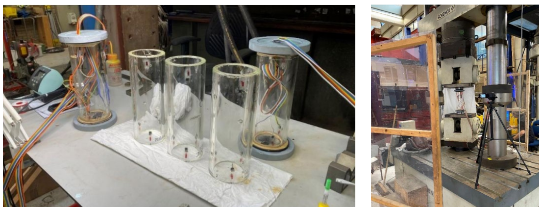
Fig 8. Left: samples ready for testing, right: one of the samples placed in the compression machine.
