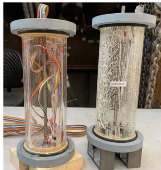
Fig 10. Left: one cracked annealed sample, right: one cracked heat-strengthened sample.
