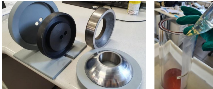
Fig 7. Left: steel and POM components, right: lamination process of one of the samples.
