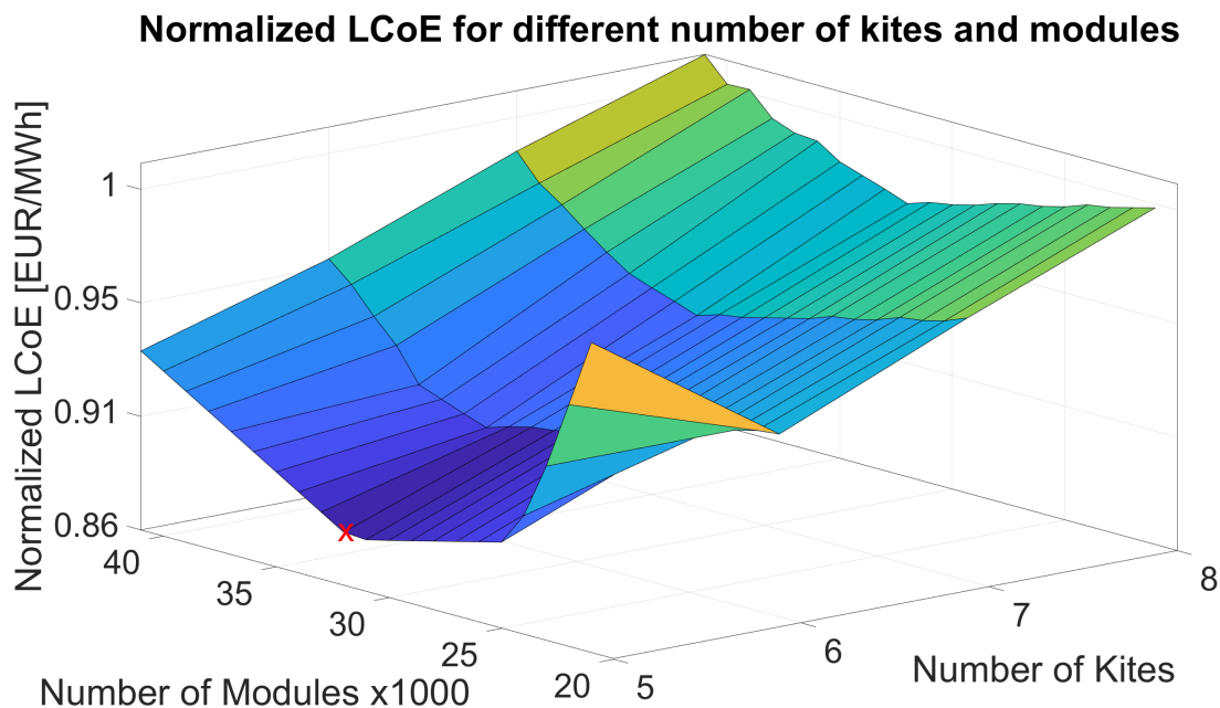
Figure 3.33: A surface plot of the LCoE, dependent on a different number of kites and modules.
