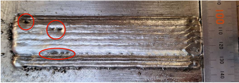
Figure 16. overlap beads deposition of Stellite 6 on top of stainless steel overlapped beads.
