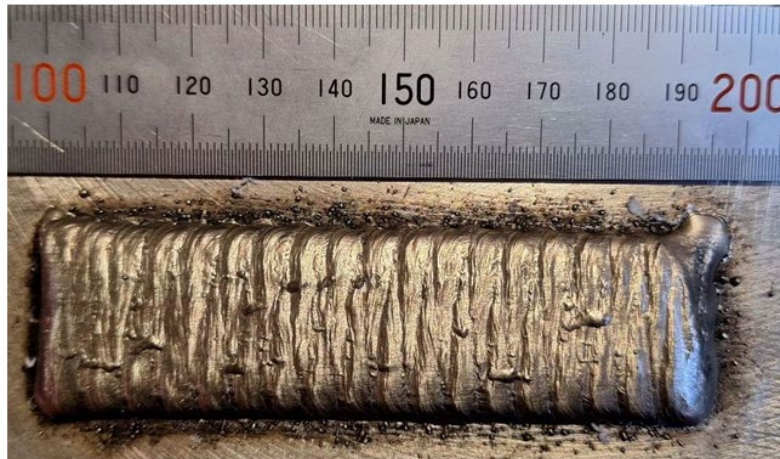
Figure 22. Overlap beads deposition of Stellite 6 on top of stainless steel deposits with oscillating depositing path
