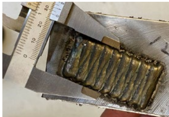
Figure 26. oscillation pattern deposited with optimal process parameters.
