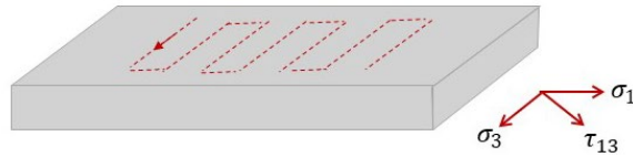
Figure 34. Schematic representation of in-plane stress components ( \sigma_1 , \sigma_3 , \tau_{13} ) aligned with the GMAW toolpath
