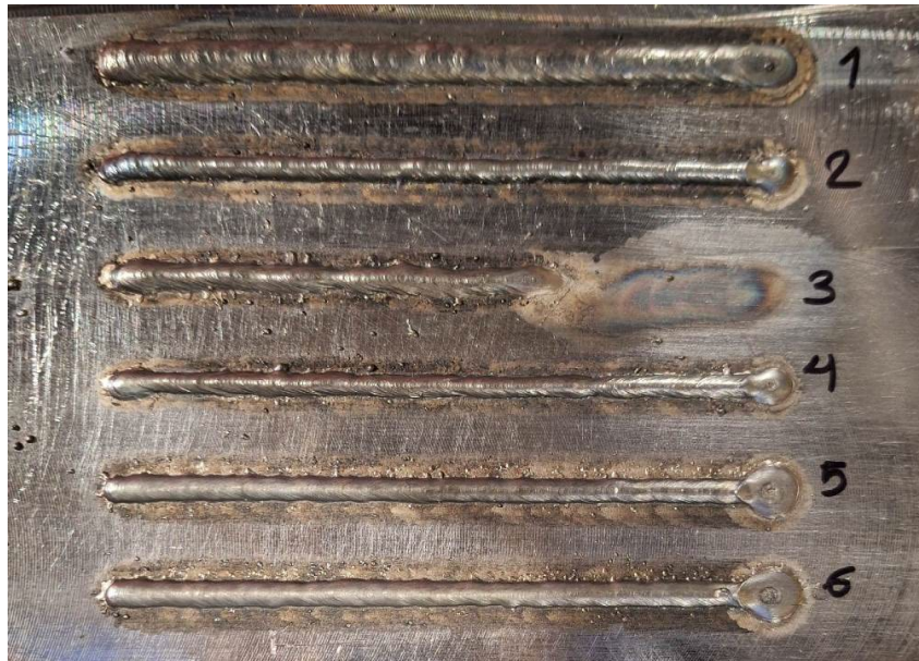
Figure 15. single bead deposition of Stellite 6 with Accu-Pulse® welding mode
