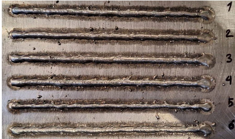
Figure 20. single bead deposition of Stellite 6 with Versa-Pulse™.
