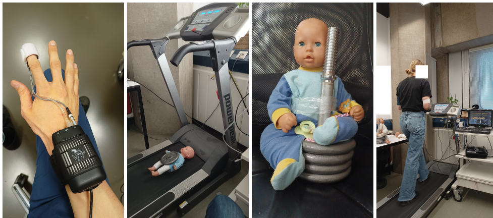
(a) Hand & finger module of Finapres. (b) The treadmill with the 5 kg doll. (c) The 10 kg doll that needs to be lifted. (d) Subject walking with Finapres.
