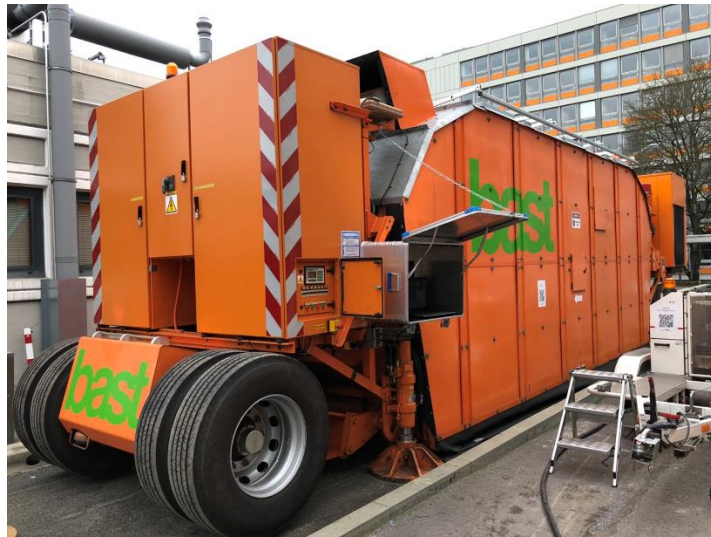
Figure 4. The APT test conducted by MLS 30
