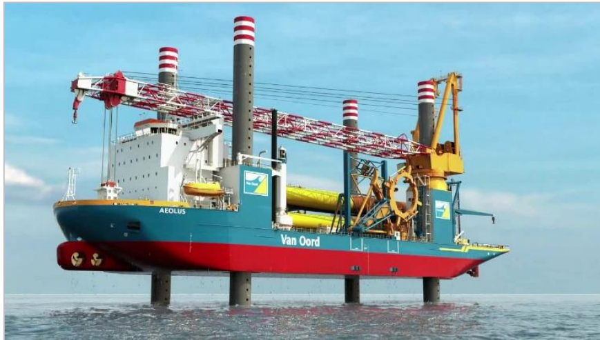
Figure 1.3 Offshore installation vessel Aeolus in jacked-up position.
