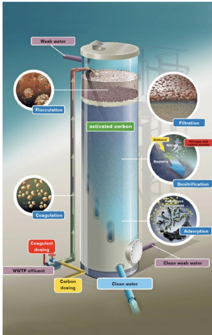
Figure 2-2 Illustration of the functions of the 1-STEP® filter
