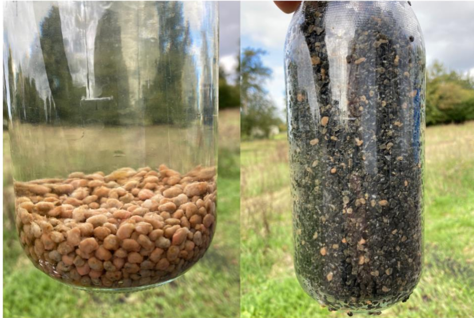
Figure 5-7 Biofilm morphology and size distribution of the granules from the aerobic zone (left) and anoxic zone (right).
