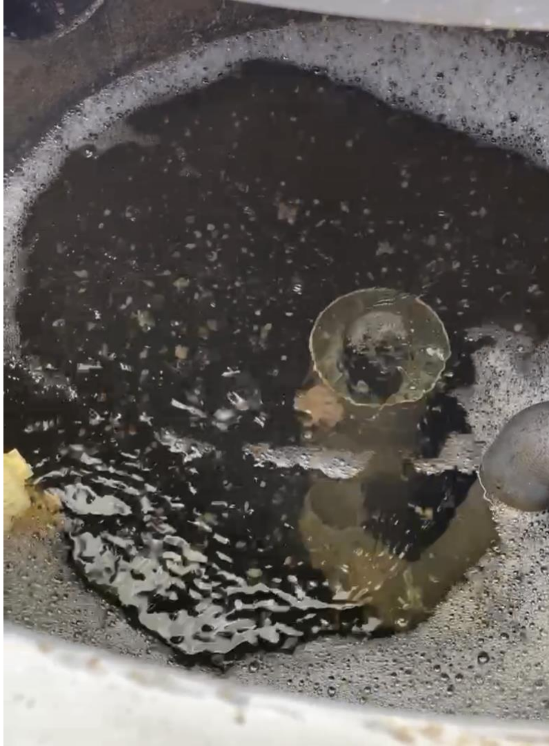
Figure 5-1 Photograph of the supernatant in the 1-STEP filter. The brown granules are biomass.
