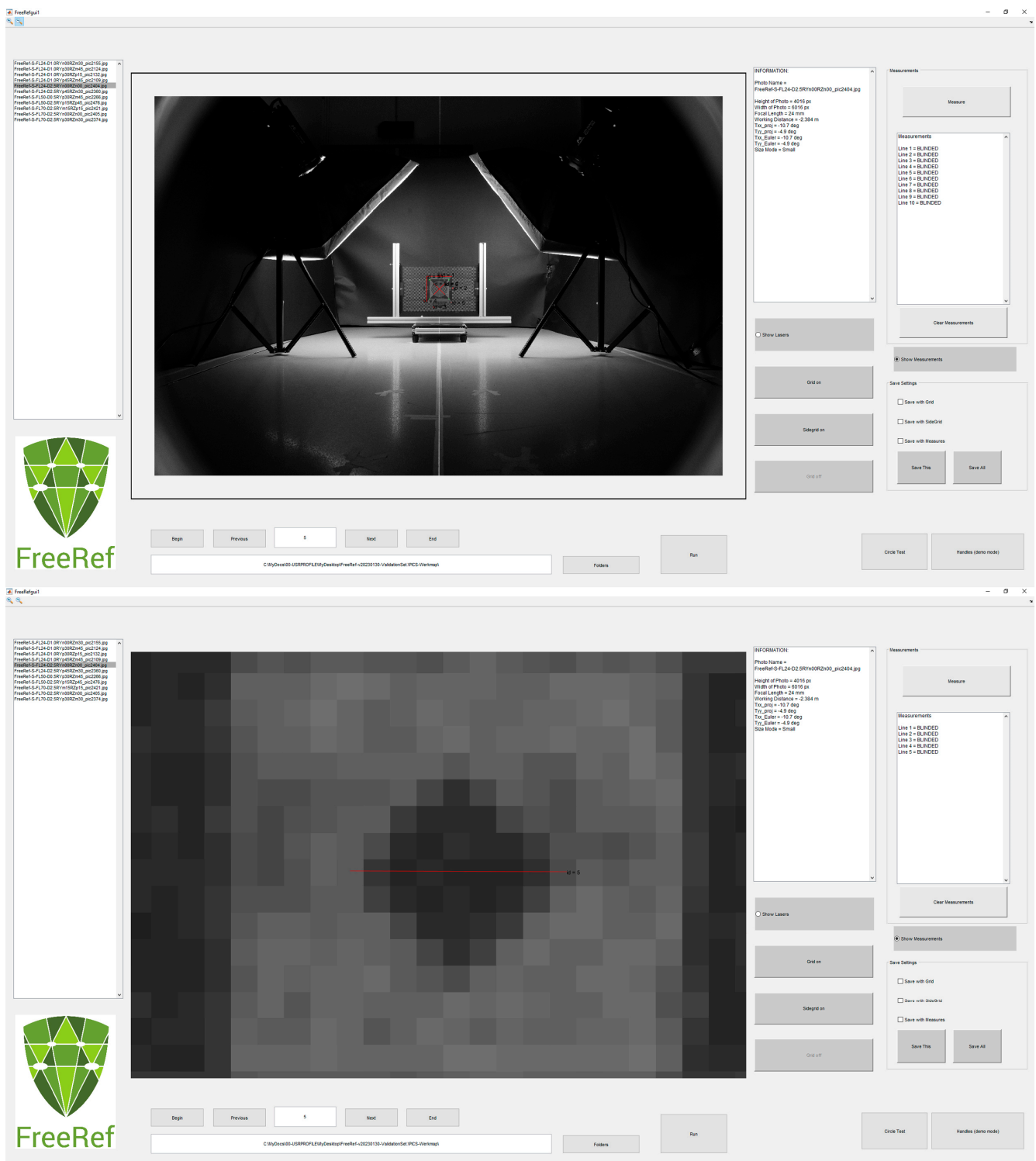
Figure 14. Example of how the measurement lines were placed in the FreeRef-1 software by the assistants. ( Top ) Interface with photo entirely zoomed out and all 10 verification line measurements shown. ( Bottom ) Interface with photo zoomed in to measure verification line number 5, showing the challenge of targeting the correct corners of the square.
