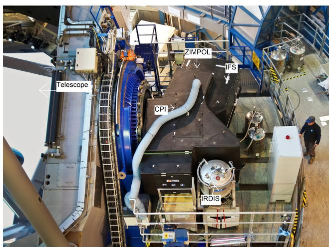
**Figure 4.1:** Picture of SPHERE on the VLT. The location of each of the instruments is labeled. Adapted from ESO instrument description.<sup>1</sup>
